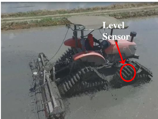
Figure1. LI data collection during final tilling (land smoothing) using level sensor
