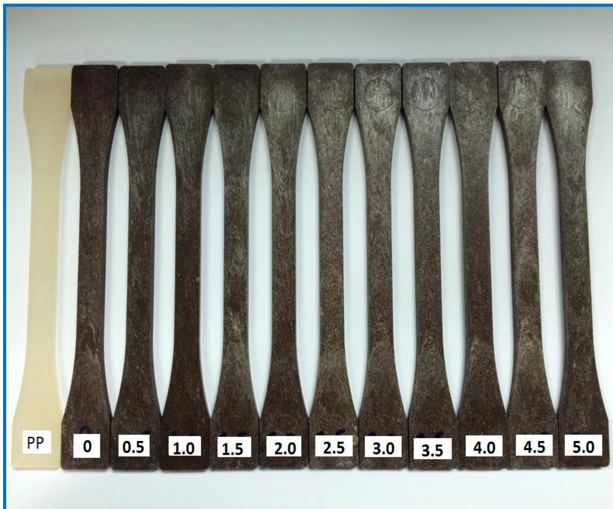
Figure 1: Images of samples made of pure polypropylene and different content of nanoclay
