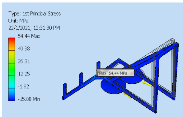
Figure 6: Value of 1st Principal Stress on the design analysis of a cabbage cutting mechanism
