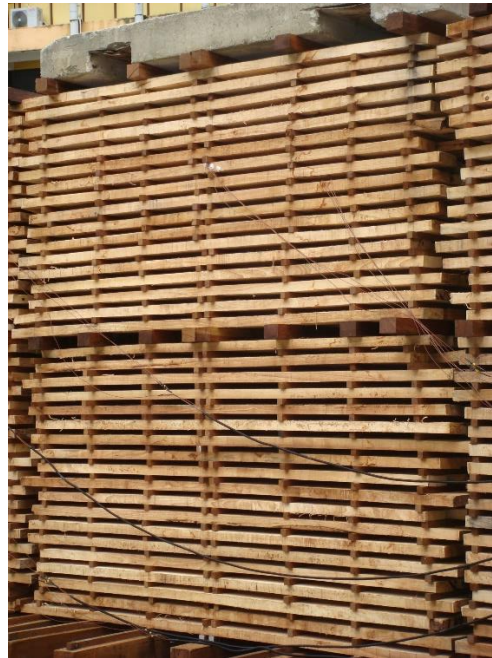
Figure 2. Sample boards with inserted thermocouples, systematically placed in within the box-stacked timber bundles at specific stack-heights.
