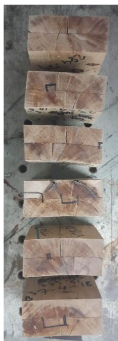
Figure 4: Bakau specimens post vacuum pressure delamination test with mixed of percentage of total delamination.
