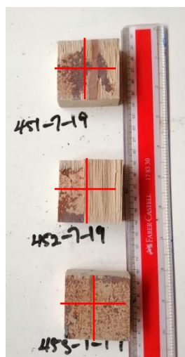
Figure 6: Bakau specimens post block shear test with low percentage of wood failures.
