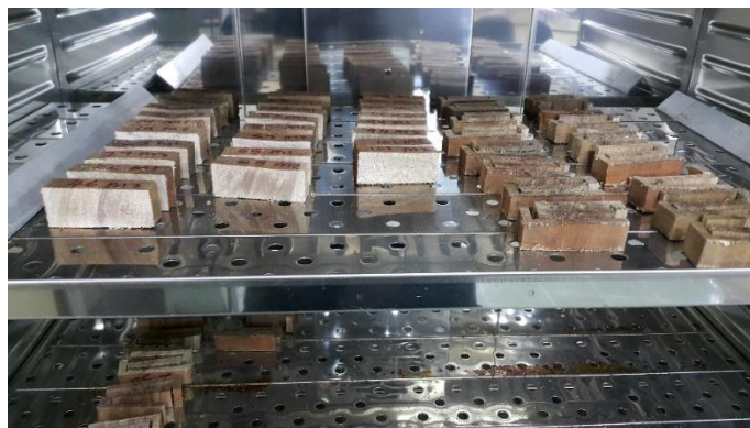
Figure 3. MC determination based on standard oven drying method.
