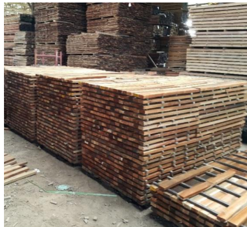
Figure 2. Stacking of timber with properly aligned stickers at specific spacing.
