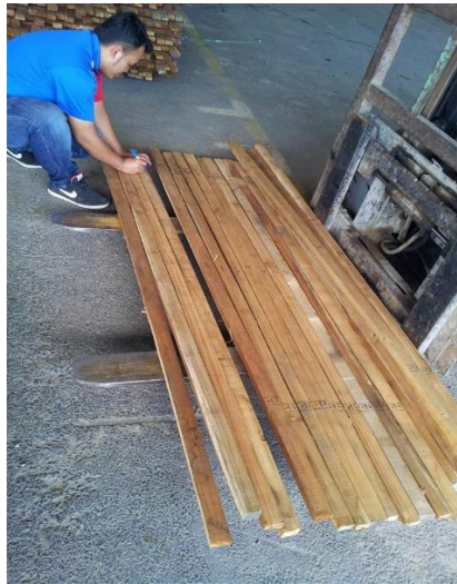
Figure 2. Stacking of timber with properly aligned stickers at specific spacing.
