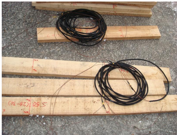
Figure 1. Sample boards from both sawn length-groups inserted with thermocouple wire for monitoring of internal wood temperature during drying process.
