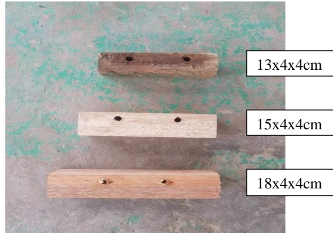
Figure 1. rectangular wooden track grousers 13x4x4cm, 15x4x4cm and 18x4x4cm
