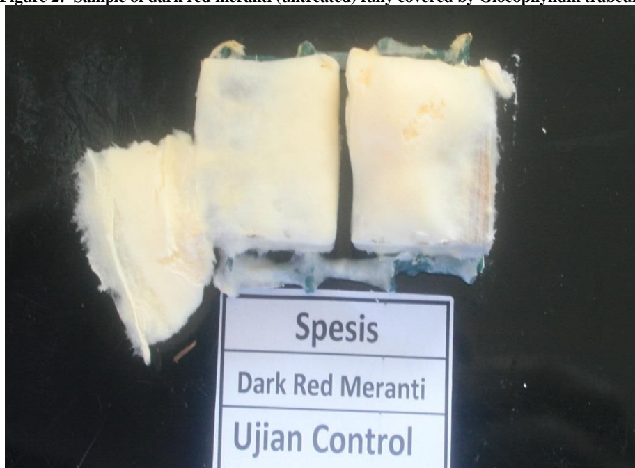
Figure 2: Sample of dark red meranti (untreated) fully covered by Gloeophyllum trabeum
