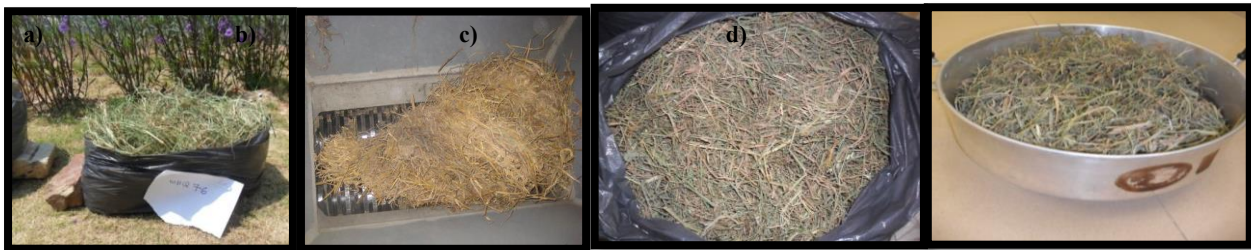
Figure 1: The process of preparation for paddy straw before pulping process a) drying paddy straw, b) paddy straw processed by crusher machine, c) paddy straw after processed, d) paddy straw ready for mix with concentration NaOH.
