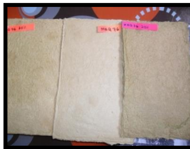
Figure 3: The sample of paper that produce from the different types of paddy straw
